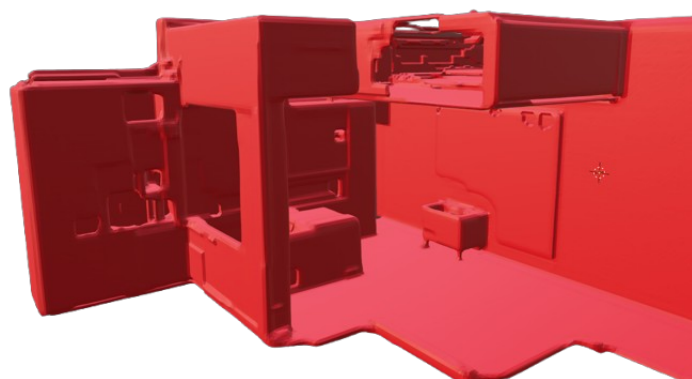
Figure 16: A picture of the mesh of area A. The rectangle is meant to represent a television, but the model has interpreted the area to be its own room. The model may have interpreted the area as a bathroom, with a sink and bathtub as potential furniture.
